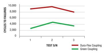
When a new, out-of-the-box, Dura-Flex coupling and a green coupling were subjected to a stop-start cycle test, Dura-Flex was 2X –100X better.
