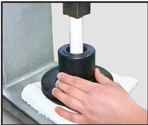
Press the bushing into place.
