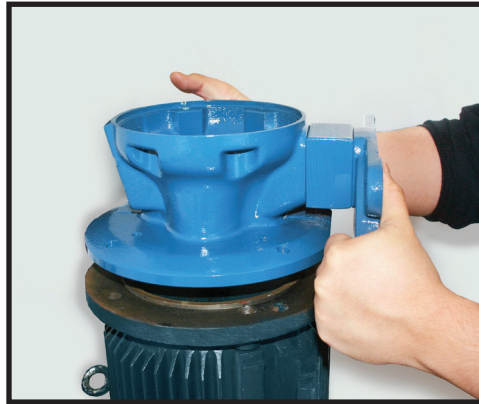
Lower the assembly onto the motor, aligning the 4 adapter holes with the 4 motor mounting holes.
