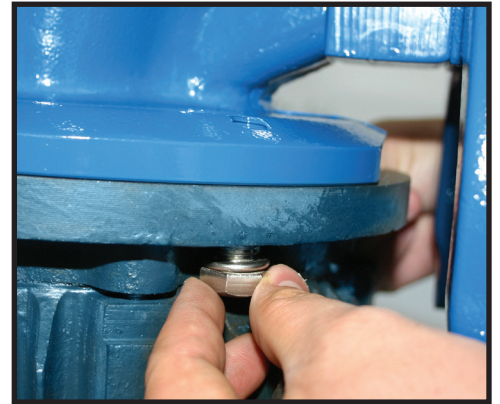
Insert and tighten the 4 bolts through the motor into the adapter.
