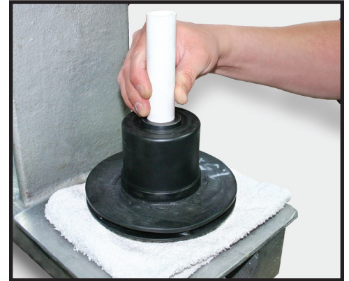
Center the PVC pipe on the bushing.
