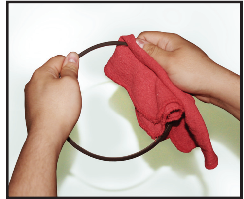
Clean and check the O-ring gasket.
