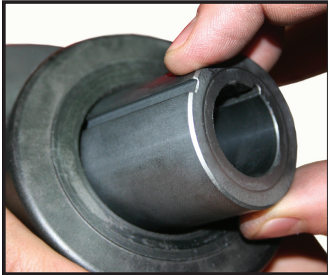
Insert the bushing. Make sure it remains aligned while inserting into the press.
