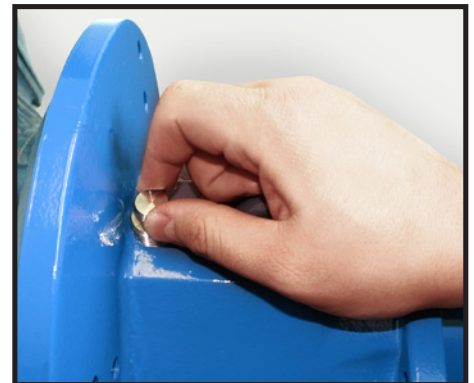
Replace the metal plug on the adapter and drive end assembly is complete.
