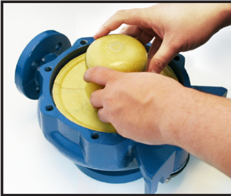
Lower the containment shell into place.
