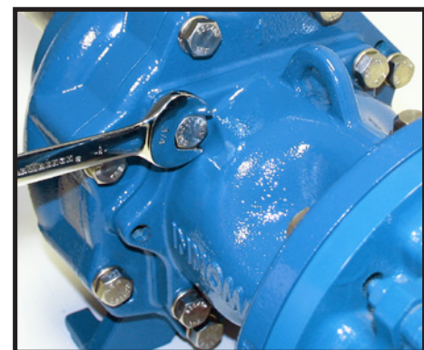
Retract the jackscrews until the two pump halves are mated. Insert and tighten the (4) adapter hex bolts to the torque given in the Torque Table on the following page.
