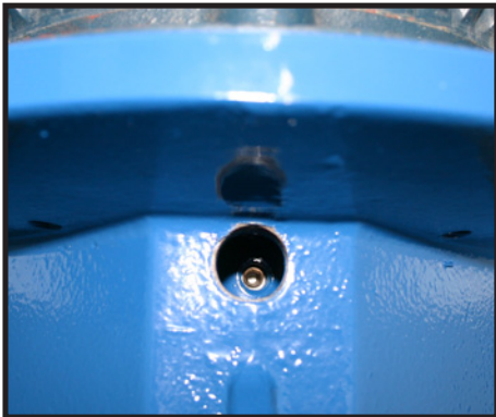
Locate the first set screw (A).
