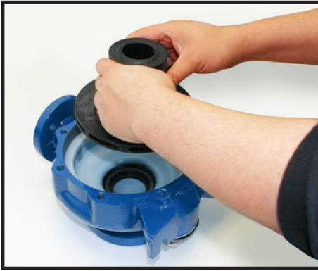
With the casing face down, insert the impeller.
