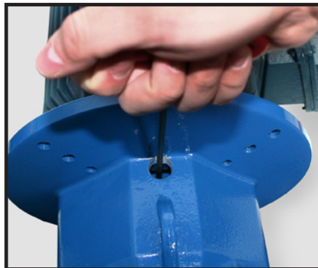
Tighten the second set screw with the T-handle allen wrench.
