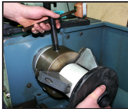
Insert the impeller into the lathe and tighten the jaws.
