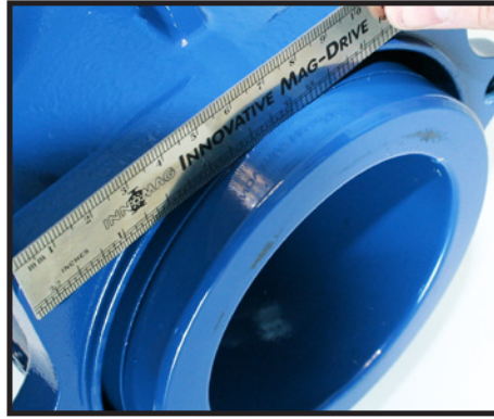
Use a ruler, straight edge or visually align the groove with the adapter.
