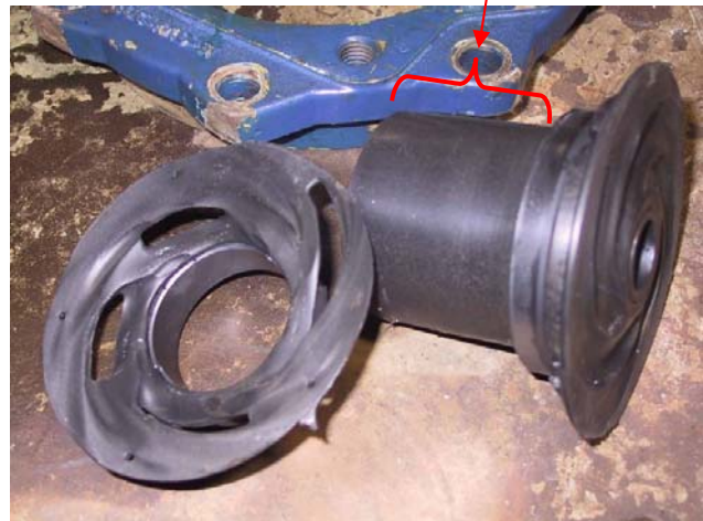
Figure 4 – No wear on magnet assembly
