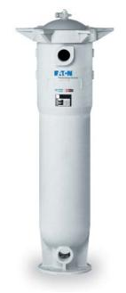
POLYLINE single bag filter housing is constructed with glass fiber reinforced polypropylene or PVDF. It features superior corrosion resistance as well as high-pressure and temperature capabilities. The POLYINE has one injection molded body meaning no seams or weak points.
