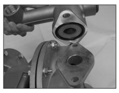
STEP 2 Remove the "Discharge Manifold".
