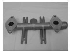
STEP 5 Remove the "Suction Manifold".
