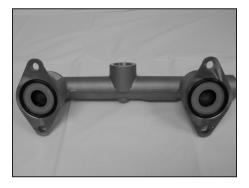
Remove the "O-Ring", "Valve Seat" and "Ball" from the "Discharge Manifold".
